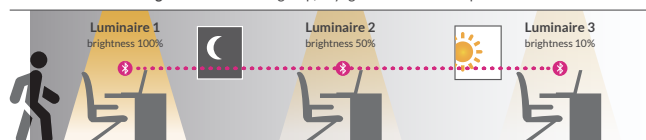
Schematic diagram 3 Luminaire group, daylight detection & compensation
